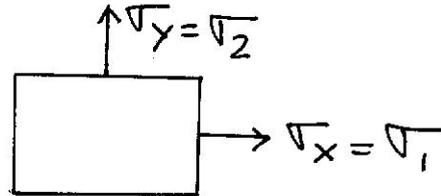
Cyl:  $\sigma_H = \frac{pD_m}{2t}$ ,  $\sigma_L = \frac{pD_m}{4t}$ ,  $\sigma_m = \sigma_H \sqrt{\frac{3}{4}}$
