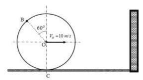
The figure shows a uniform disc of mass 5 kg, and radius 2 meter. It rolls without slipping with a forward velocity of its center O at a velocity of  $10 \, m/s$ .
